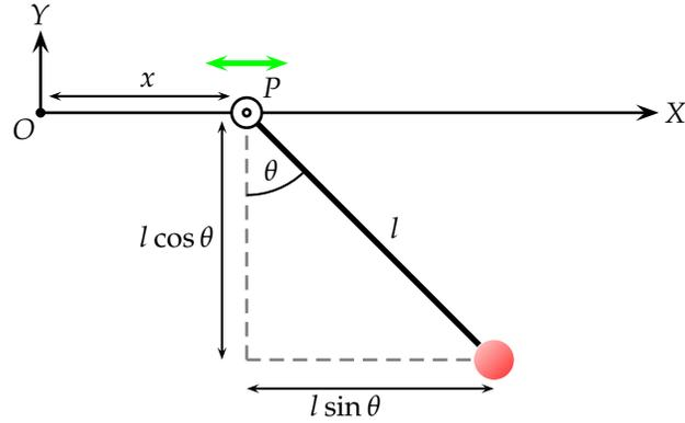
Figure 1: Coordinate set up for establishing the Lagrangian for the driven simple pendulum where the pivot is constrained to move along the X-axis. | Drawing by AD.
