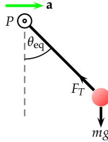
Figure 3: Diagram for deriving the expression (2) for the equilibrium angle ( $\theta_{\text{eq}}$ ) when the pivot of the pendulum moves at a constant acceleration where the sign convention is:  $\vec{a} : (+) \mid \overleftarrow{a} : (-)$ , so that the equilibrium angle is positive if the pendulum is to the right of the downward vertical, and negative if it is to the left of the downward vertical. The tension on the pendulum mass is  $F_T$ . | Drawing by AD.
