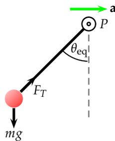
Figure 2: When the pivot moves at constant acceleration  $\mathbf{a}$  to the right with respect to an inertial frame, the pendulum settles at an angle  $-\theta_{eq}$ ; that is, to the left of the downward vertical. The horizontal force component of the tension force ( $F_T$ ) on the pendulum provides the necessary force on the pendulum mass to achieve the rightward acceleration  $\mathbf{a}$ . | Drawing by AD.
