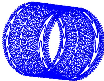
Figure 6: Phase portrait of the simple pendulum whose pivot point is driven according to  $\ddot{x} = -\Omega^2 x$ . The phase portrait is the same as in that shown in Figure 5 but with the time dimension also added in. The two-dimensional circular cross section in the (angle, angular velocity) phase space then becomes the three-dimensional cylinder in the (angle, angular velocity, time) space.
