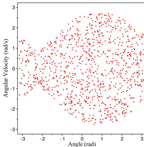
Figure 8: The Poincaré section for the simple pendulum whose phase portrait is depicted in Figure 7. Unlike the regularity seen in the Poincaré section in Figure 5, we see that the pendulum may return to the same angular position with respect to the downward vertical but its angular velocity is not guaranteed to have the same magnitude as it had before in an earlier cycle. The phase points show a sense of randomness on the Poincaré section.
